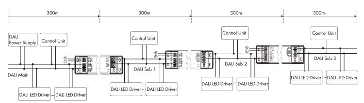
Note: In case of series wiring, up to 3 repeaters can be connected and the DALI bus can be extended up to 1200 meters.
